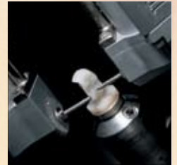
The milling unit carves the ceramic restoration in about 15 minutes.
